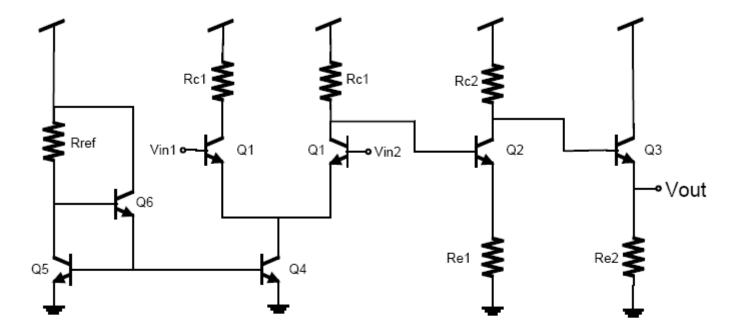
Current source: Determine  $R_{ref}$  for desired currents in differential amplifier (Lect. 15)
